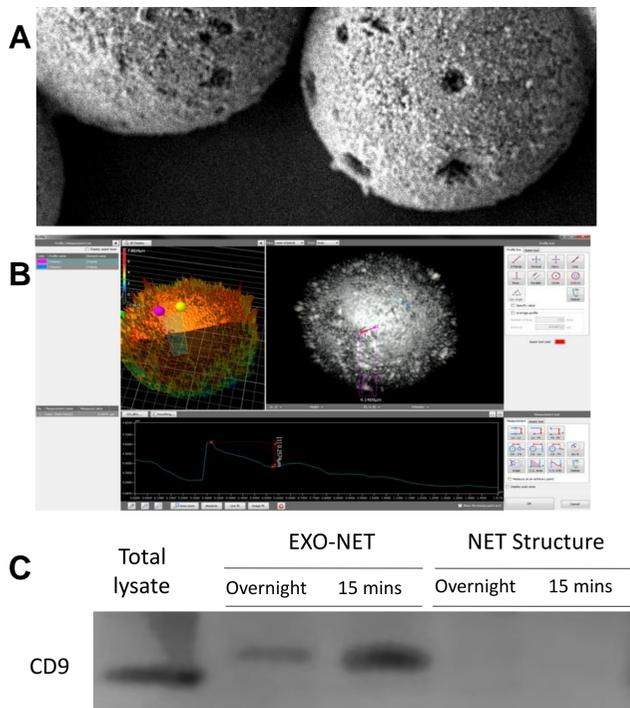
**Figure 1. (A)** Scanning electron micrograph showing ultra-structure of the EXO-NET™ matrix, including pores, coated on 2.5 um magnetic particles.
